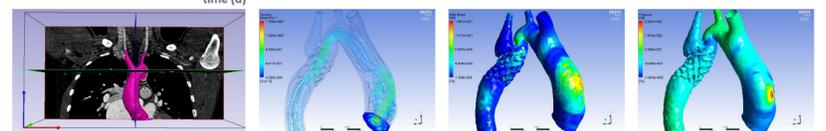
**Figure 3:** CFD models using finite-element volumetric meshing methods were used to simulate aortic hemodynamics for pulsatile flow. Several flow characteristics, including flow streamlines and wall shear stress, were calculated for three cardiac cycles.
