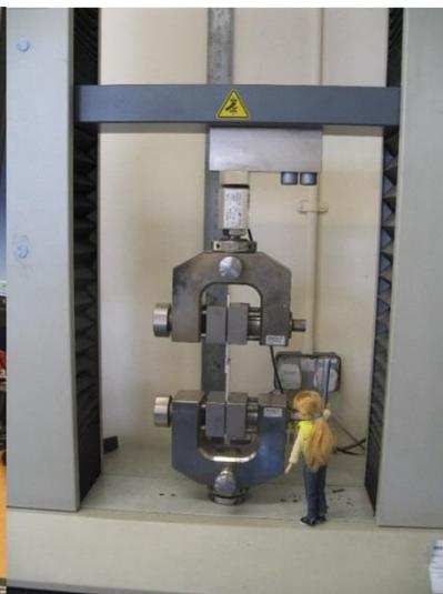
Here Lottie is inspecting the CAD CAM drawings for a part and then conducting a tensile strength test. This is testing the bond between two pieces of metal to make sure it is strong enough to be part of a car.
